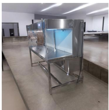
LuxMed® Horizontal Laminar Airflow Cabinet LM-LAFH-200 Series are designed to provide clean air environment for research operation which required complete anti-bacterial working area. The series involves constant positive pressure inside the cabinet which prevents intake of contaminated air.
